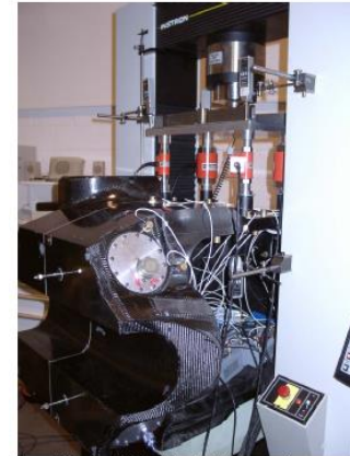
Figure 11 Showing A23 chassis in side static squeeze rig
