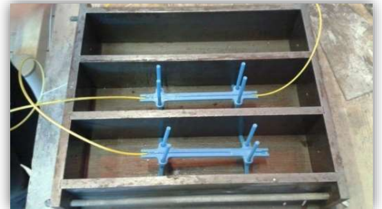
Image 2&3 : 1D Fiber Optic Sensor Prismatic Sample Setup
