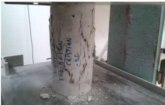
Image 5: Compression test on a non-instrumented sample
