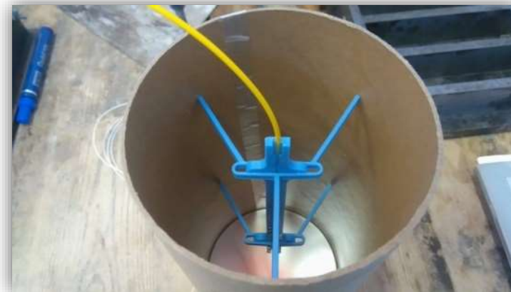
Image 4 : 1D Fiber Optic Sensor Cylinder Sample Setup
