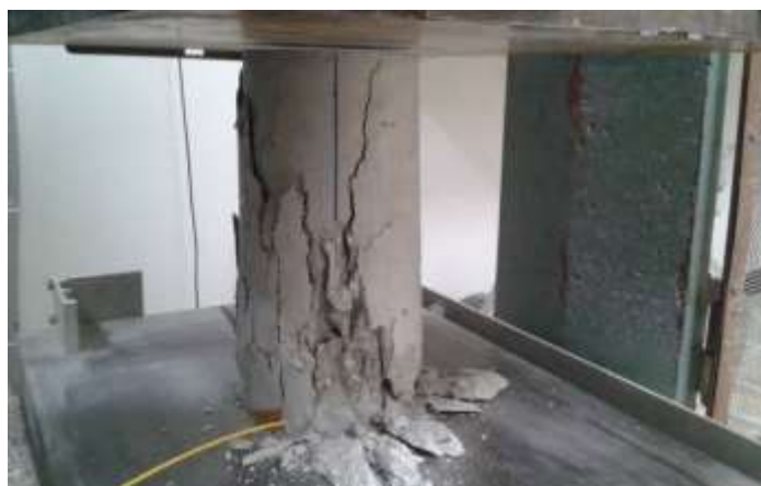
Image 6: Compression test on a instrumented sample
