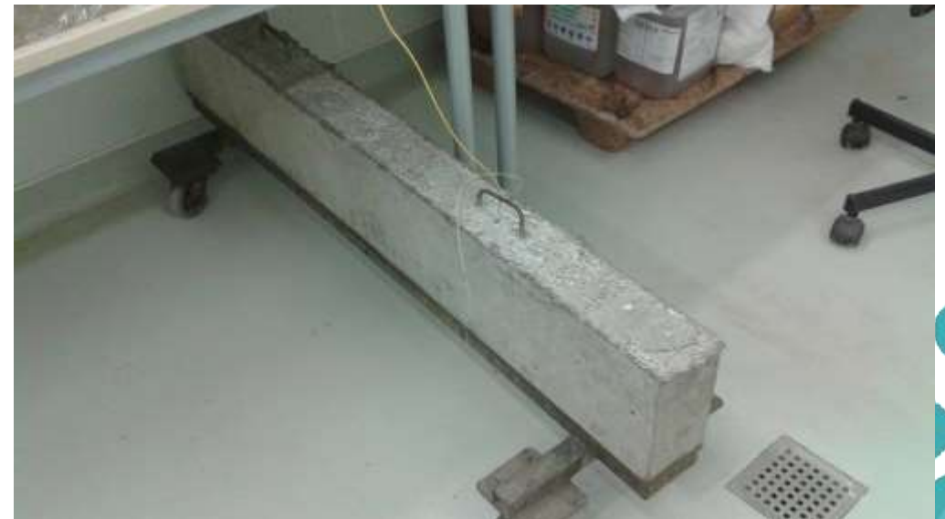
Image 15: Experimental Setup for the shrinkage measurements
