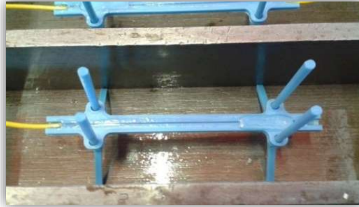
Image 2&3 : 1D Fiber Optic Sensor Prismatic Sample Setup
