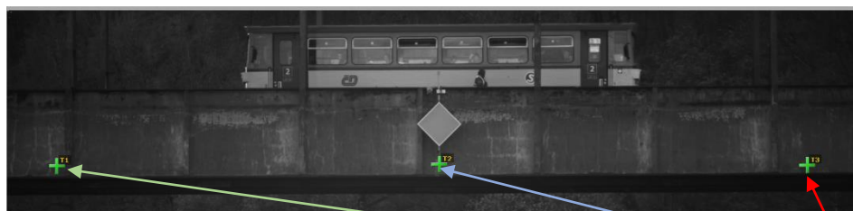
Pic 13: deflection of the bridge on three points
