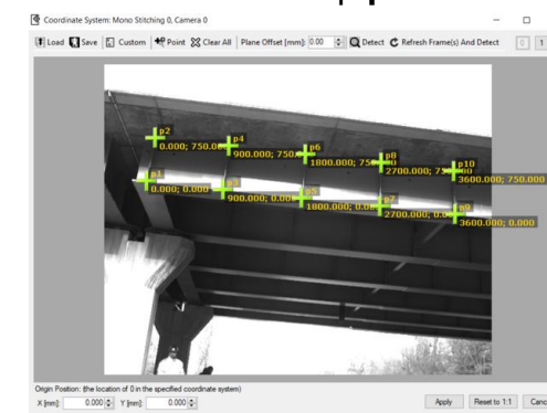
Pics 14: calibration using known dimensions of the bridge
