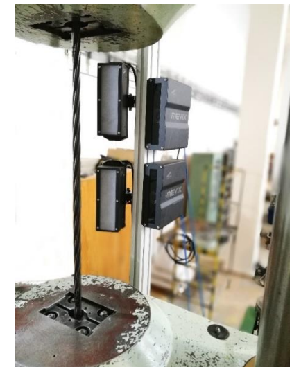
Pic 15: 2 cameras for long Field Of View
